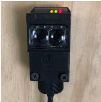
Photo-eye with 10-foot maximum range
