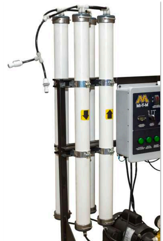
Fresh-water reverse osmosis membranes with permeate outlet and sampling port
