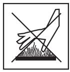
Serious injury may occur from touching the electrical motor. This area can remain hot for some time after the Biological Recycling System is shutdown. Never allow any part of your body to contact the electrical motor until cooled.
