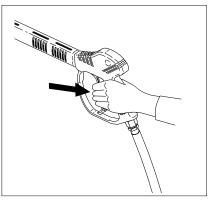
**STEP 2:** Trigger the spray gun to eliminate trapped air then wait for a steady flow of water to emerge from the spray wand. Then install nozzle.
